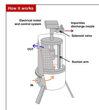
**Filtration.** Filtration is achieved through a multi-layer screen. As soon as the filter screen is clogged, a pressure switch detects the pressure difference between inlet and outlet and starts the cleaning cycle.
