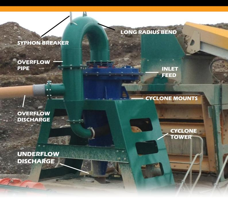
Overflow pipe work should be manufactured from the pipes specified in the table below. It should also include a syphon breaker vented to atmosphere also as specified in the table. The overflow pipe should be independently supported and should not hang from the cyclone. Flanges are PN16 and details for inlet and overflow flanges can be found at the end of this brochure.
